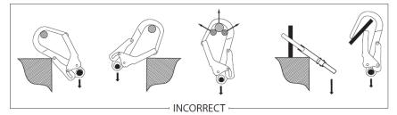
• It is necessary to protect the snap hook gate with locking gear. - See drawing.
