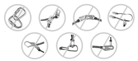
\* Rollout: A process by which a snap hook or carabiner unintentionally disengages from another connector or object to which it is coupled. (ANSI Z359.0-2007)
